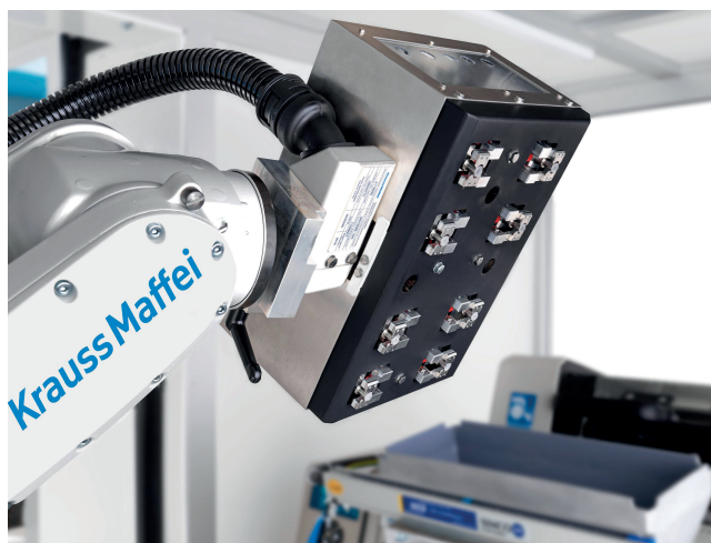
Fig. 2. Combination gripper for membrane slitting and parts removal
